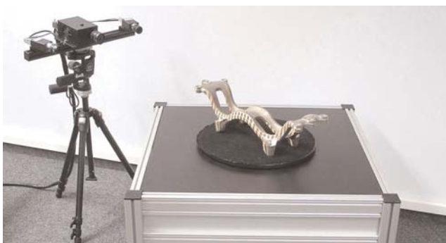
Program controlled Rotary Device for automated data acquisition
